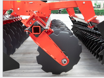
Individual Rubber Disc Suspension
